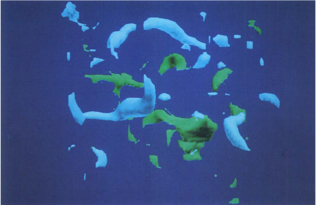
FIGURE 26. Direct numerical simulation ( 128^3 resolution points) corresponding to figure 25(a). The blue surfaces delimit regions where the pressure p verifies p_{min} \leq p \leq 0.36 p_{min} . The green surfaces bound the regions within which the absolute value of the scalar fluctuations is larger than 41% of the instantaneous maximum.
